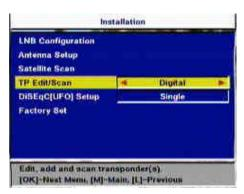
In this menu you can scan through the transponders for specific channels, e.g. when new channels are offered in the package of a specific broadcaster. You can obtain this information from the corresponding video text or TV and satellite magazines. You can choose between "analogue" and "digital".
